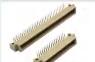
欧式插座弯公系列 Spec: Din 41612 Male Connector Right Angle Series Positions: 2X16/2X32 pin Installation type: Right angle through hole soldering
