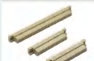
欧式插座直母系列 Spec: Din 41612 Female Connector Straight Series Positions: 2X5/2X8/2X10/2X16/2X20/2X32 pin Installation type: Through hole soldering
