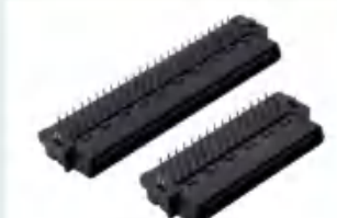
SCSI全型90°系列 Spec: SCSI Screw-Type 90° Connector Series Positions: 20~100 pin Installation type: Right angle through hole soldering
