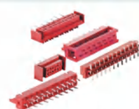
1.27mm IDC压线头 Spec: 1.27mm IDC Crimping Type Connector Positions: 4~26 pin Installation type: Through hole soldering/ Puncture & assembly wire type
