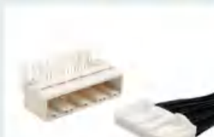
2.2mm信号连接器(平齐款) Spec: 2.2mm Signal Connector Positions: 8~40 pin Installation type: Through hole soldering
