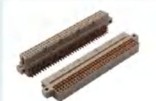
欧式插座三排弯母 免焊型 Spec: Din 41612 Connector 3 Row Press-fit Type Positions: 96 pin Installation type: Through-hole crimping
